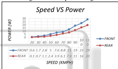
Fig. 9: comparison of front and rear bumper readings in series connection
