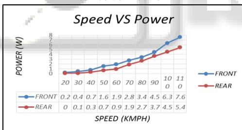
Fig. 10: comparison of front and rear bumper readings in parallel connection
