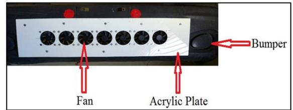
Fig. 4: front bumper assembly with attached fans
