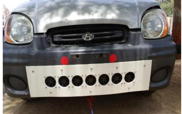
Fig. 5: actual view of the front bumper assembly
