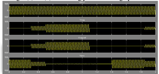
Fig.6. Voltage sag compensation in proposed system
