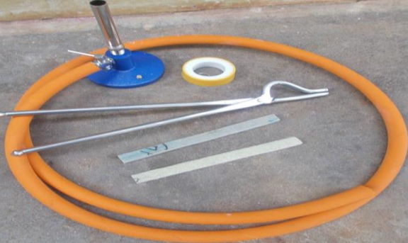
Fig. 3: Gas burner clamped with cylinder tube
