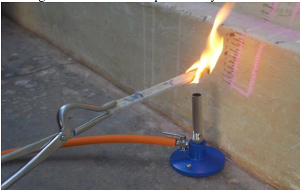
Fig. 5: Polyester specimen exposed to fire retardant laminates test
