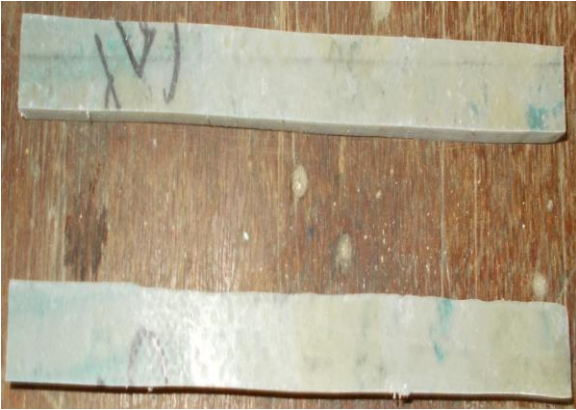
Fig. 1: Polyester specimens for fire retardant laminates test
