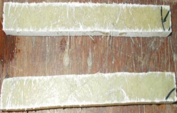
Fig. 2: Epoxy specimens for fire retardant laminates test
