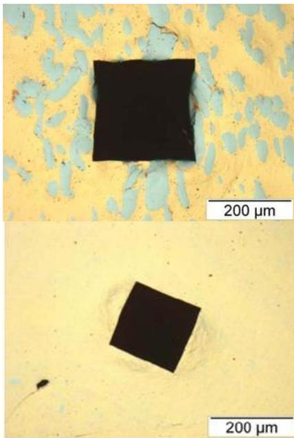
Fig. 8: Hardness measurement on cross sections of bulk CuCr 75/25 (upper photo) and on the molten top layer of CuCr 75/25 after making and breaking tests (lower photo); Cr grains have a grey colour.
