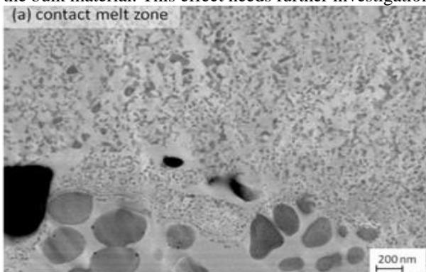
Fig. 9: Microstructure of the molten layer on top of the contact surface (re-solidified). The chromium grain size is in the range of 200 nm; in addition fine-dispersed chromium exists [6].
