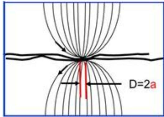
Fig. 3: Scheme of contact point between the surfaces of two flat contacts. The contact point is assumed to be a sphere.
