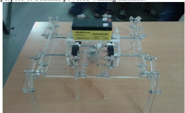
Fig. 1: Eight leg mechanism of walking robot
