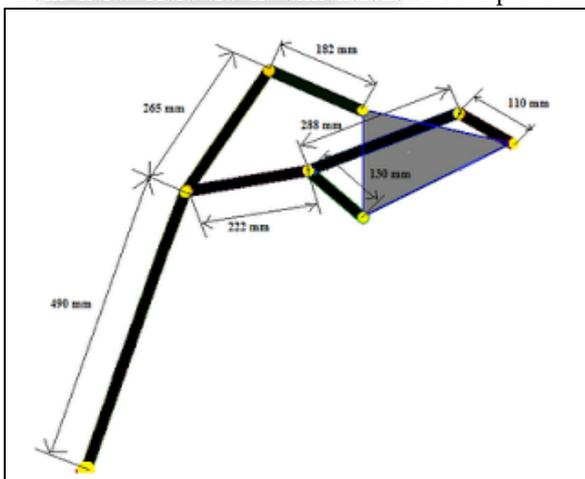
Fig. 7: Linkage Dimensions
