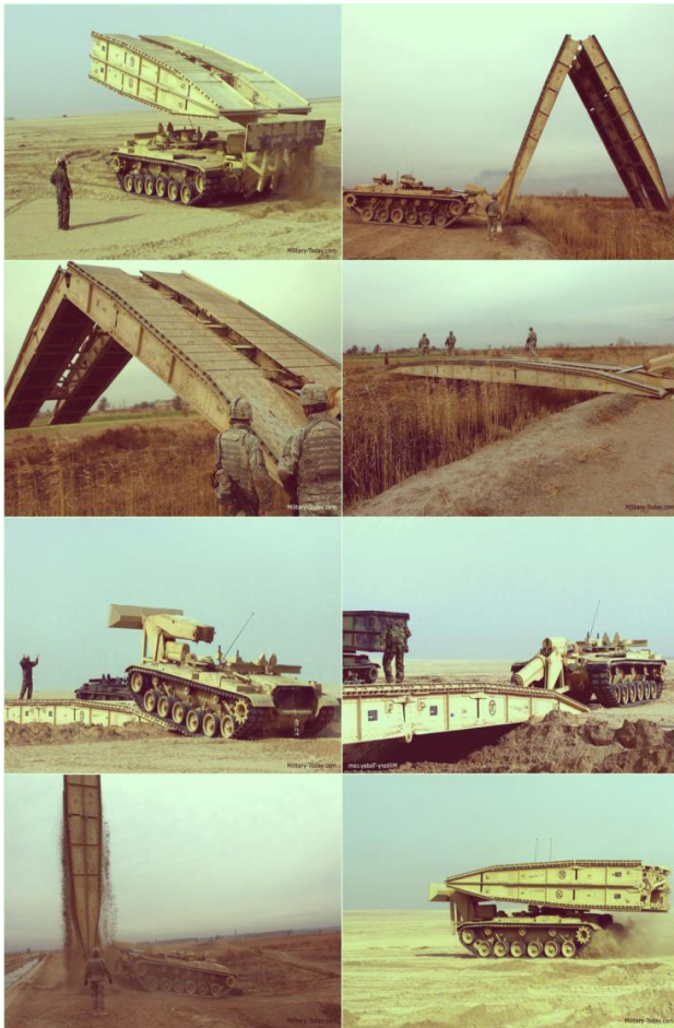
Fig. 2: Working of AVLB
