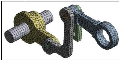
Fig. 2: FE model of linkage
