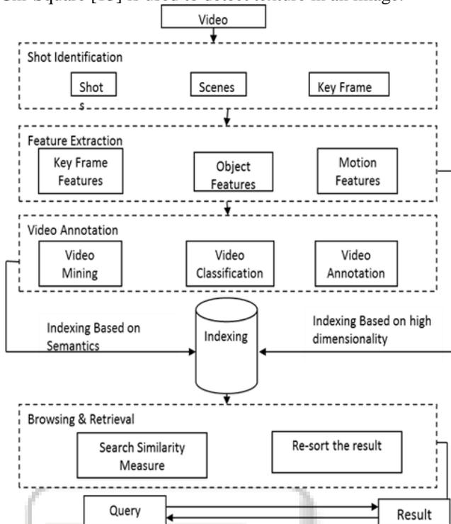
Fig. 1: Block Diagram of CBVR
