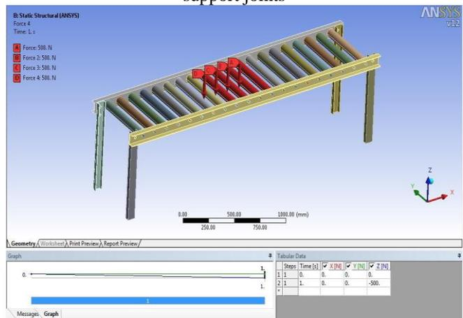
Fig. 9: A static load of 2000 N (approx 200 kg) is applied on the 4 rollers at the centre.
