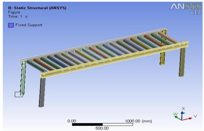
Fig. 8: Boundary Conditions - Fixed support at 4 legs and at support joints
