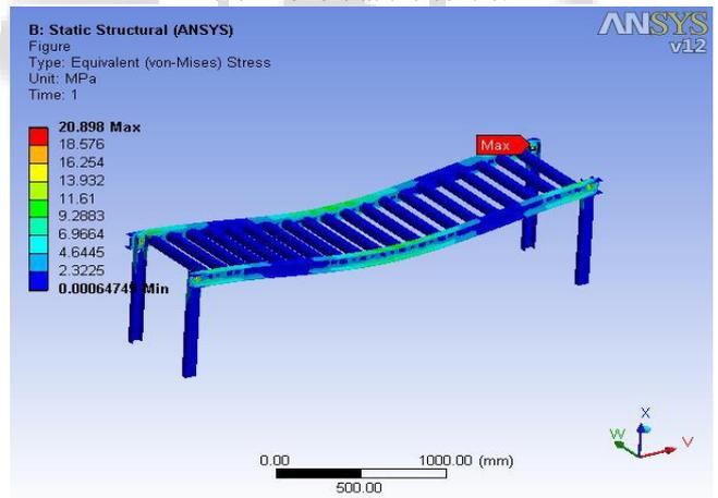
Fig. 10: stress plot for existing design
