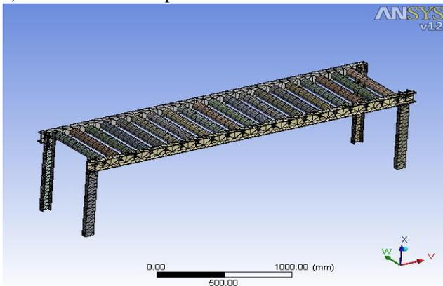
Fig. 7: Finite element mesh of the model (Isometric view)
