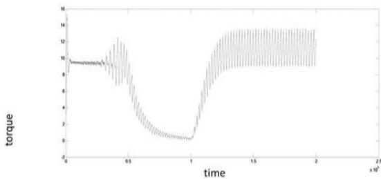
Fig. 7: Output torque of BLDC motor at no load
