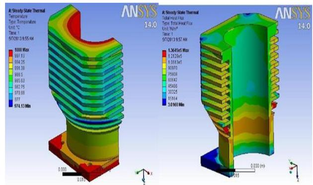
Fig. 3(a): Temperature Distribution of Cylinder Head, 3(b) Heat flux distribution
