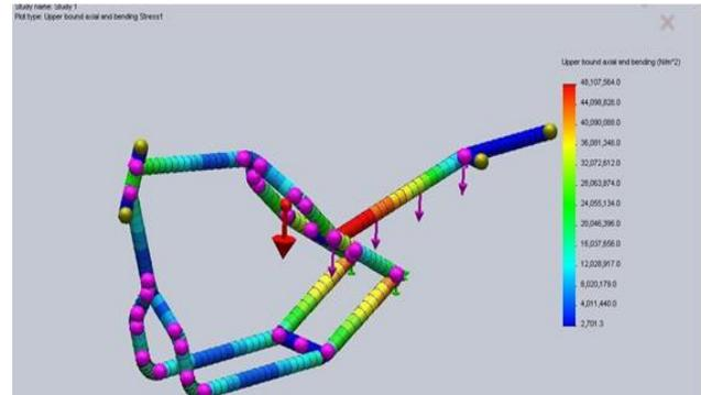
Fig. 4: Stress analysis of chassis
