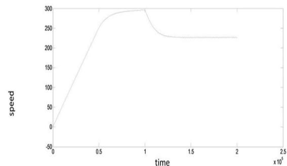
Fig. 6: Speed of BLDC motor at no load
