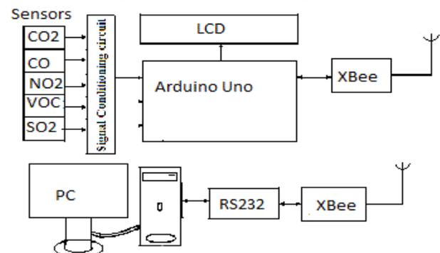
Fig. 1: Block Diagram of Indoor Air Pollution Monitoring System
