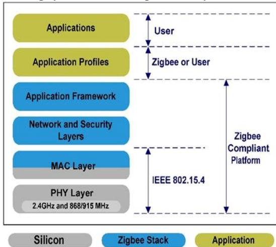
Fig. 2: ZigBee Architecture
