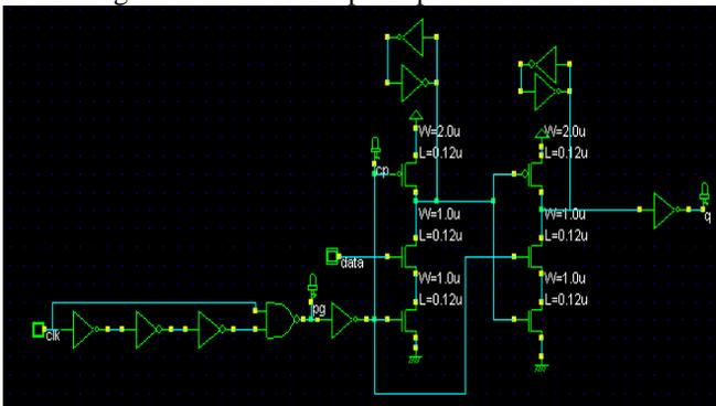
Fig. 2: Explicit pulse Data Close to out
