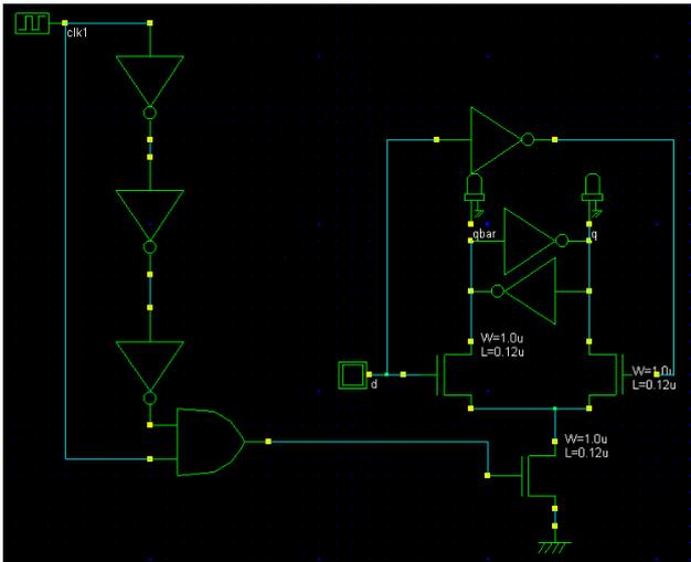
Fig. 4: Static differential sense amp shared pulse latch
