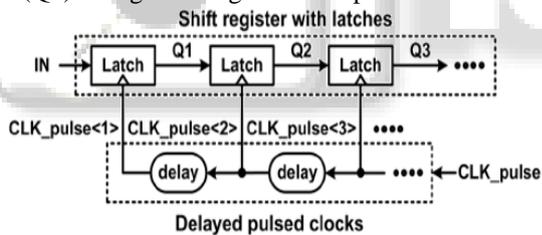
Fig. 6: Shift register with delayed clocked Latches
