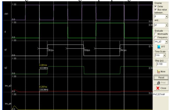
Fig. 10: Proposed 4 bit shift register design result
