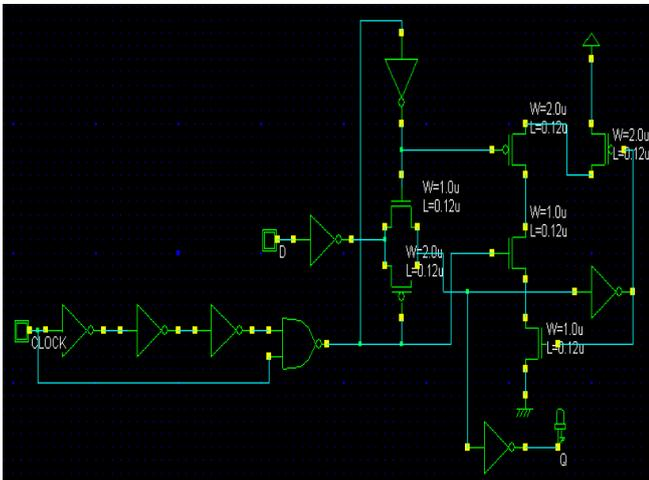
Fig. 3: Transmission Gate Flip Flop Design
