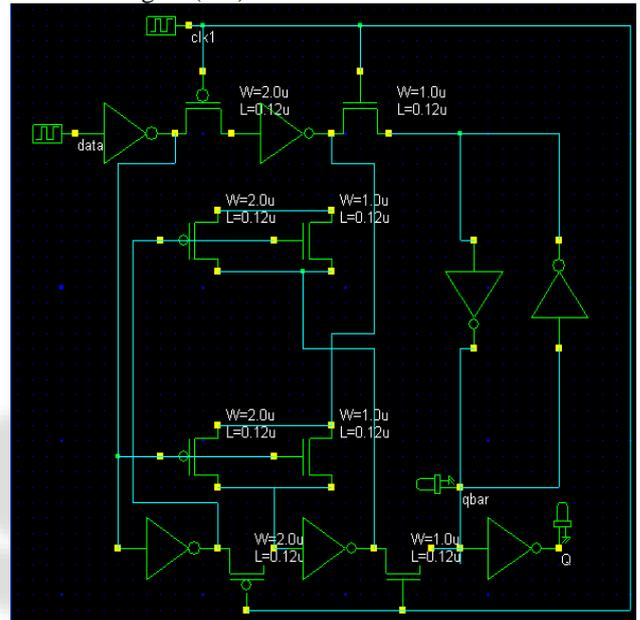
Fig. 3: Adaptive coupling Redundant Flip flop
