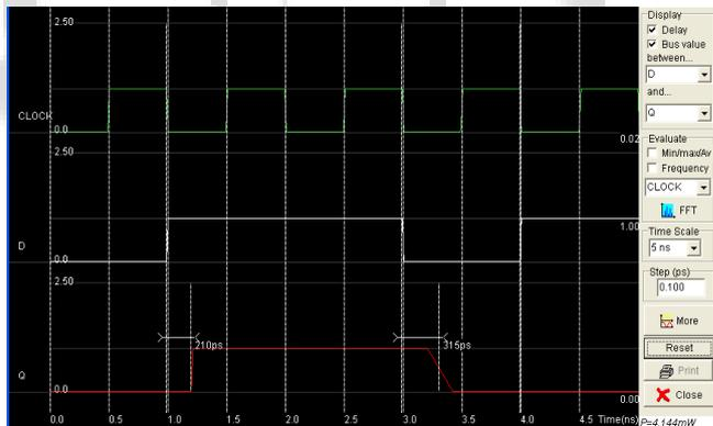
Fig. 9: Transmission gate flip flop design result
