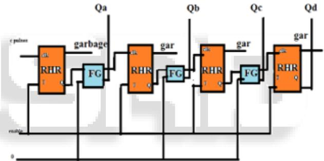
Fig. 8: Block Diagram of the asynchronous down counter
