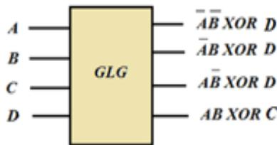
Fig. 4: Block Diagram of the GLG Gate
