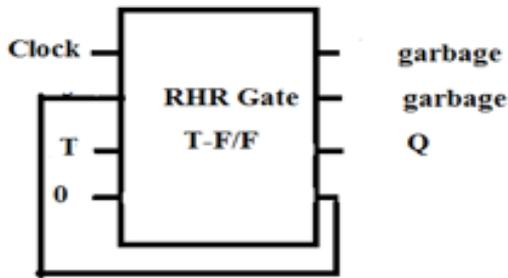
Fig. 6: Proposed T Flip flop using RHR Gate
