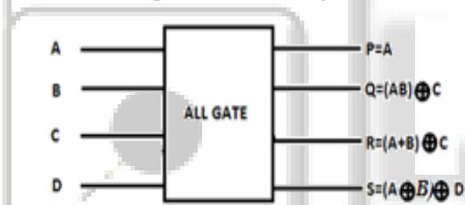
Fig. 3: Block diagram of ALL GATE
