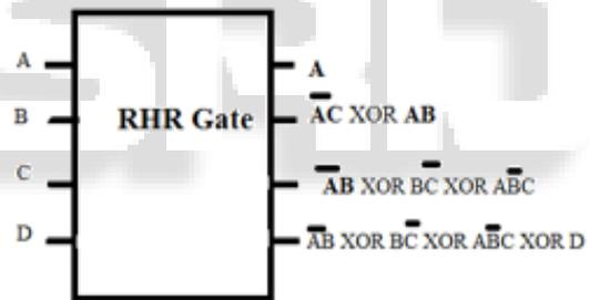
Fig. 5: Block Diagram of the RHR Gate
