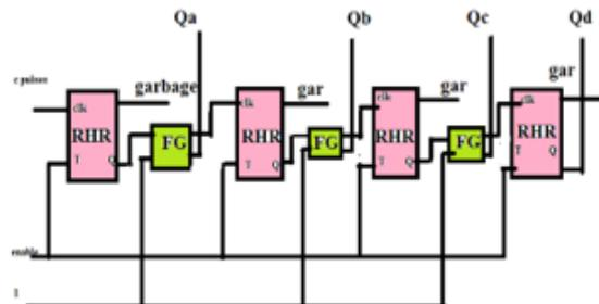
Fig. 9: Block Diagram of the asynchronous up counter
