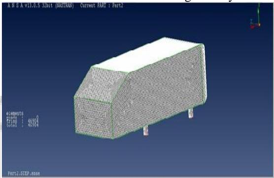
Fig. 3: Surface Mesh on Ahmed body
