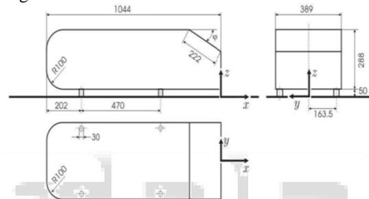
Fig. 1: Ahmed body with different slant angles (all dimensions in mm)
