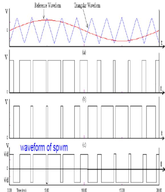
Fig. 3: Waveform of bipolar switching pulse
