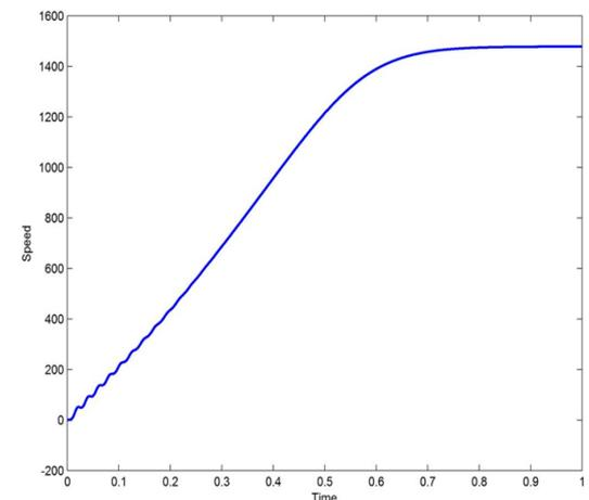
Fig. 15: Simulated result of speed time curve of unipolar PWM inverter fed three phase induction motor
