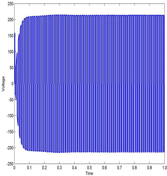
Fig. 11: Simulated result of output waveform of Bipolar PWM inverter
