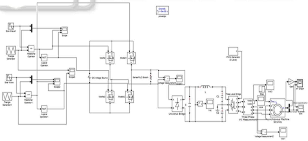
Fig. 10: Bipolar PWM inverter fed Three Phase induction Motor
