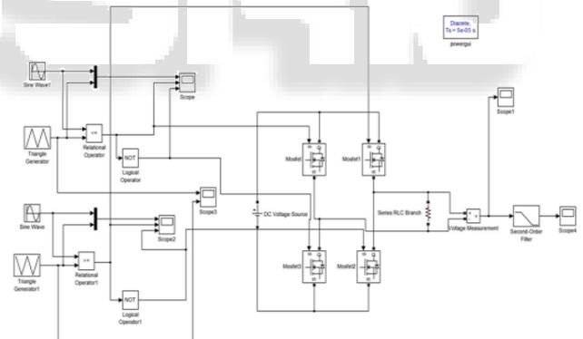
Fig. 7: Simulink modal of Unipolar PWM inverter
