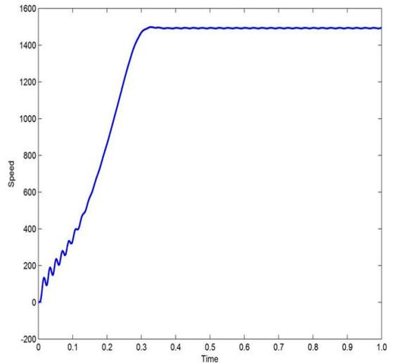
Fig. 14: Simulated result of speed time curve of bipolar PWM inverter fed three phase induction motor
