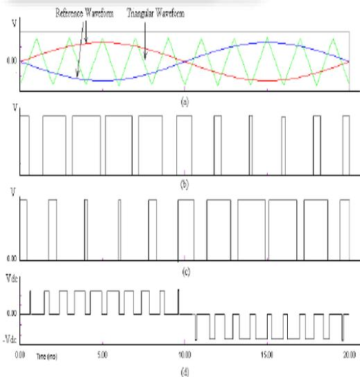
Fig. 5: Unipolar switching signal Waveform
