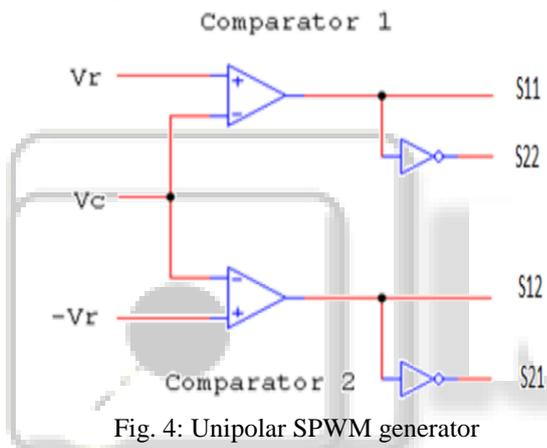
Fig. 4: Unipolar SPWM generator
