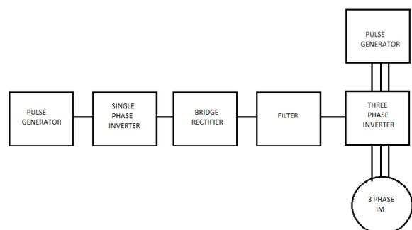
Fig. 8: Block diagram of PWM inverter fed three phase Induction motor
