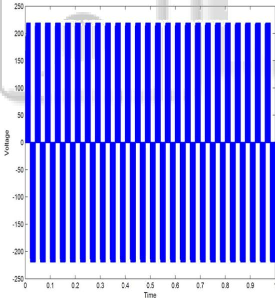
Fig. 12: Simulated result of output waveform of Unipolar PWM inverter
