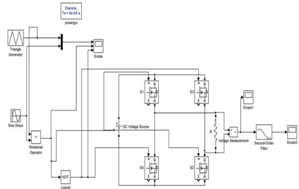
Fig. 6: Simulink modal of Bipolar PWM inverter
