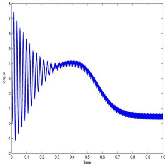
Fig. 16: Simulated result of torque-time curve of unipolar PWM inverter fed three phase induction motor
