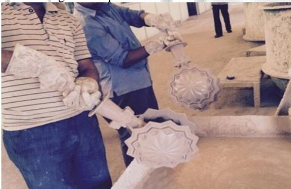
Fig. 8: Manual dipping of 1st Coat [5]
