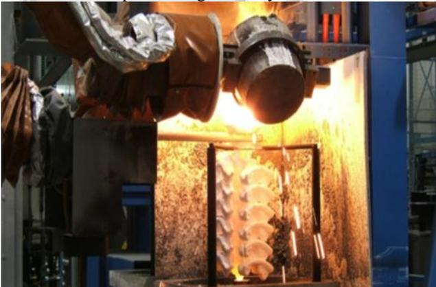
Fig. 12: Example of Automated Pouring <sup>[13]</sup>
