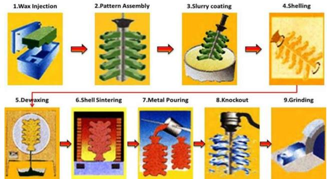
Fig. 1: Process Steps in Investment Casting Process [1]
