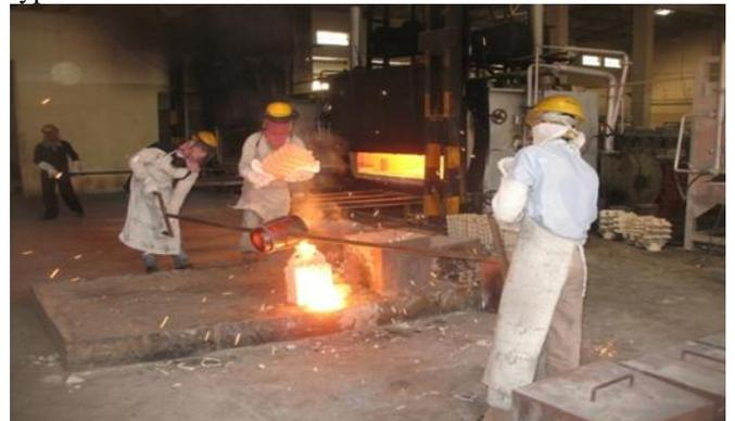
Fig. 10: Manual Pouring From Ladle to Mold
