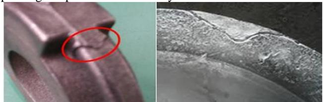
Fig. 4 & 5: Examples of Cold Shut [12]
