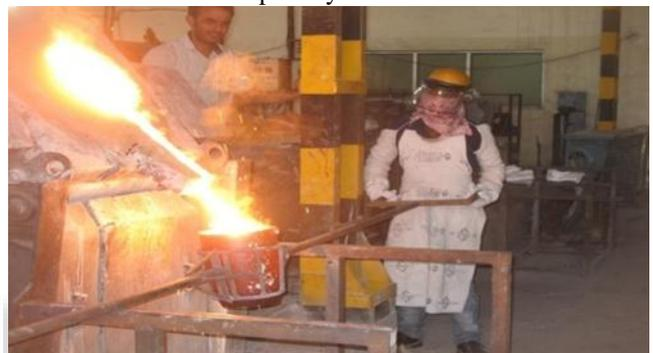
Fig. 9: Manual Pouring into Ladle [5]
