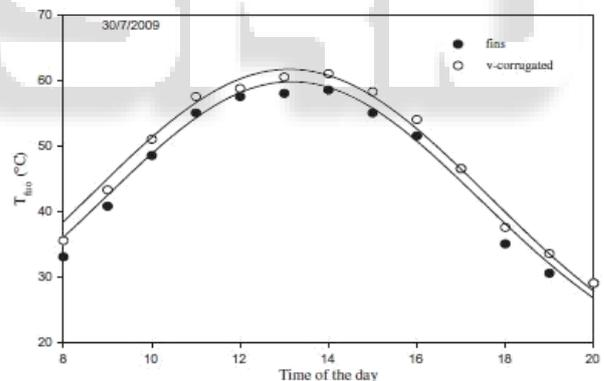
Fig. 2: Outlet Temperature of DPSAH
