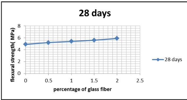
Fig. 14: variation in flexural strength according to % of glass fiber (Grade M-30)
