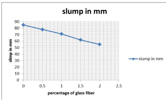
Fig. 18: slump value according to % of glass fiber (Grade M-30)
