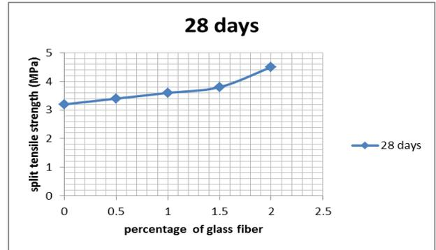
Fig. 16: variation in split tensile strength according to % of glass fiber (Grade M-30)
