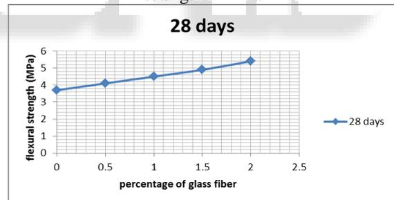
Fig. 13: variation in flexural strength according to % of glass fiber (Grade M-25)
