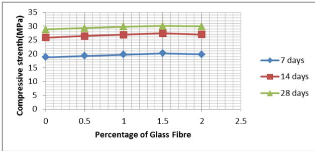
Fig. 11: variation in compressive strength according to % of glass fiber (Grade M-25)
