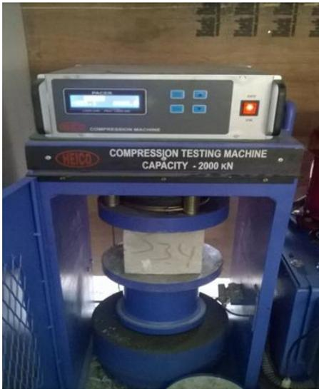
Fig. 8: Compressive Testing Machine
