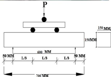
TWO POINT LOADING SETUP IN FLEXURE TEST
