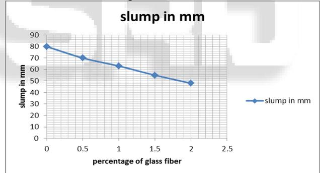
Fig. 17: slump value according to % of glass fiber (Grade M-25)
