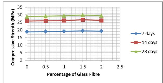
Fig. 12: variation in compressive strength according to % of glass fiber (Grade M-30)
