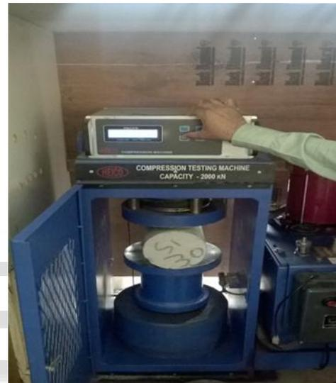
Fig. 10: split test cylinder
