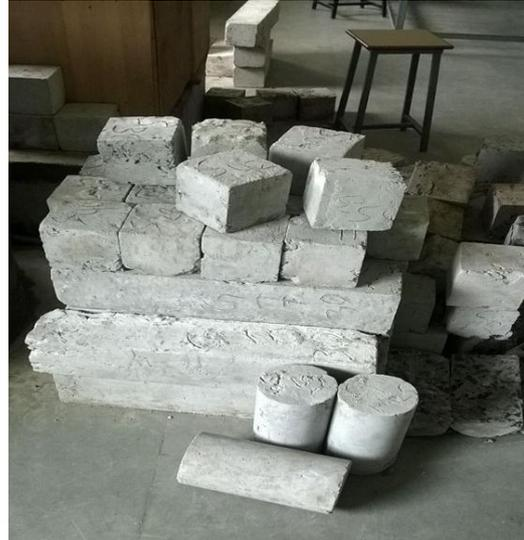
Fig. 6: casting of cubes, beams & cylinder
