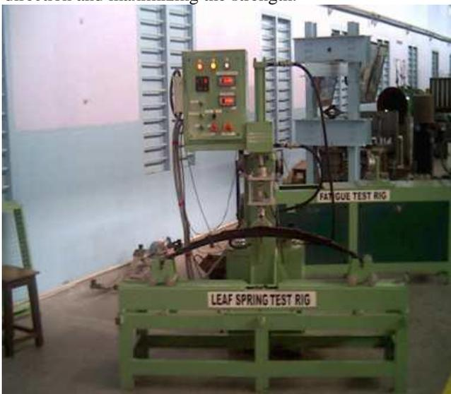
Fig. 6: Electro-hydraulic leaf spring test rig. [8]
