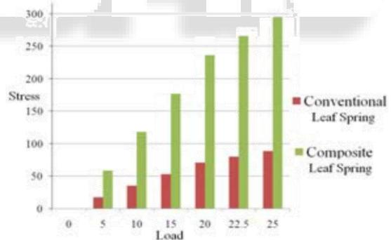
Fig. 8: behavior of the leaf springs when subjected to load and its effect on Stress. [9]
