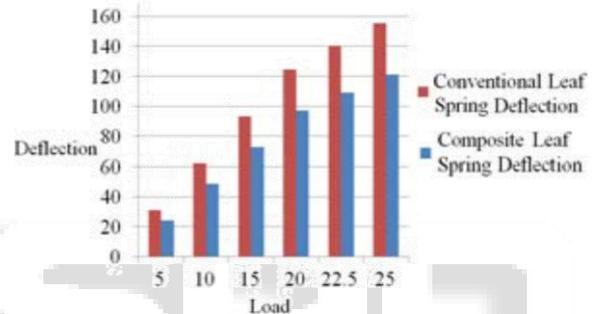
Fig. 7: behavior of the leaf springs when subjected to load and its effect on Deflection [9]
