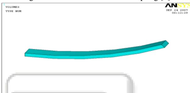
Fig. 5: Solid Model of E-Glass/Epoxy Mono Composite Leaf Spring [7]
