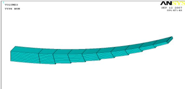
Fig. 4: Solid Model of Steel Leaf Spring [7]
