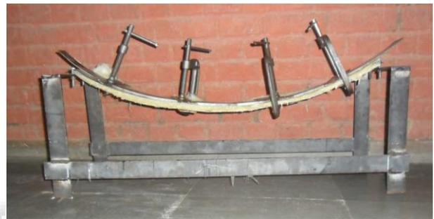
Fig. 1: E-glass/ Epoxy composite leaf spring curing on the mould set up [1]
