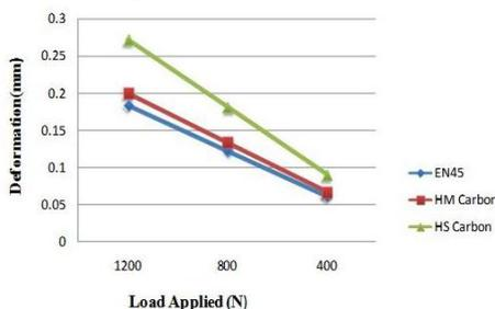
Fig. 2: Deformation at various Loads for Different material [4]
