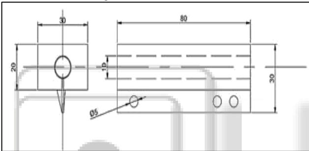
Fig. 3: Aluminium Nozzle
