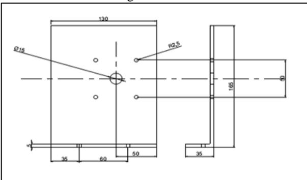
Fig. 5: Acrylic Stator Cover
