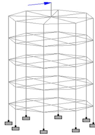
Fig. 5: Application of load on staging for calculation of stiffness
