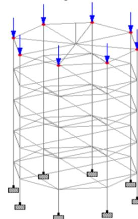
Fig. 3: Application of tank load on staging
