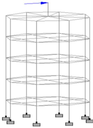
Fig. 4: Application of base shear
