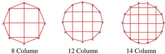
Fig. 2: Plan configuration for various number of column for frame type of staging
