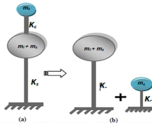
Fig. 1. Two mass model for elevated tank
