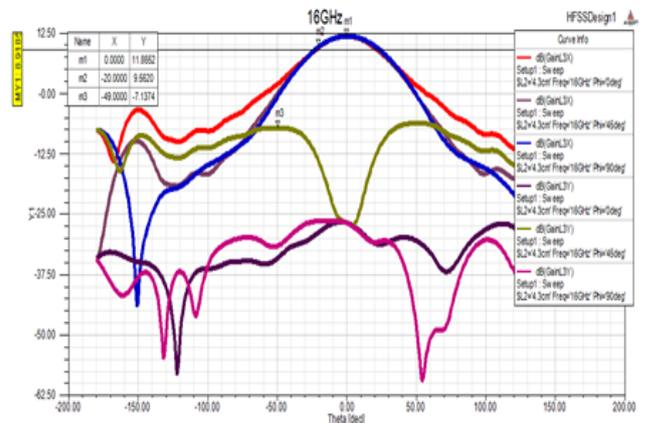
Fig. 9: Radiation pattern at 16 GHz
