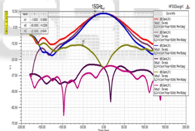
Fig. 8: Radiation pattern at 15 GHz
