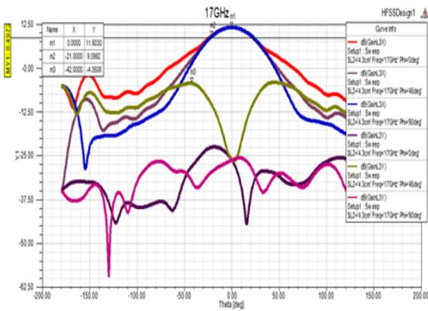
Fig. 10: Radiation pattern at 17 GHz
