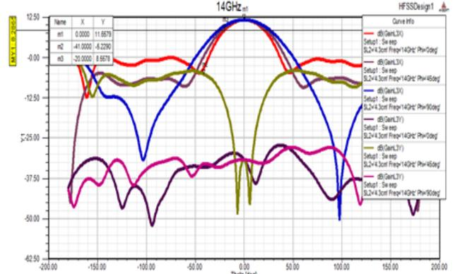
Fig. 7: Radiation pattern at 14 GHz
