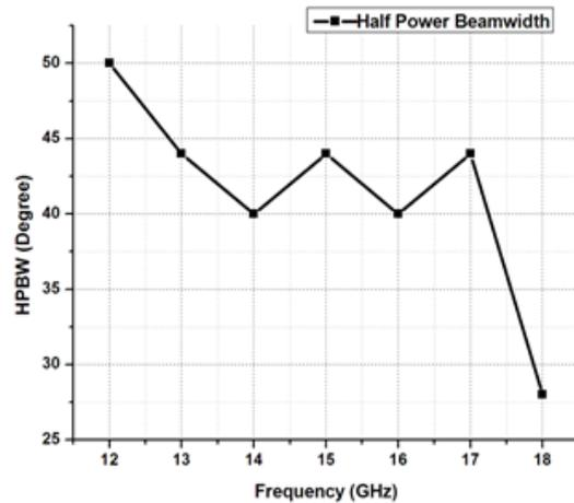
Fig. 13: Frequency vs. HPBW graph. It represents the value of HPBW at different frequency. With the increase in frequency, the value of HPBW decreases.
