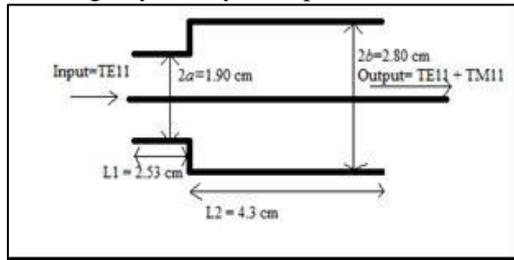
Fig. 1: Design of Step Discontinuity
