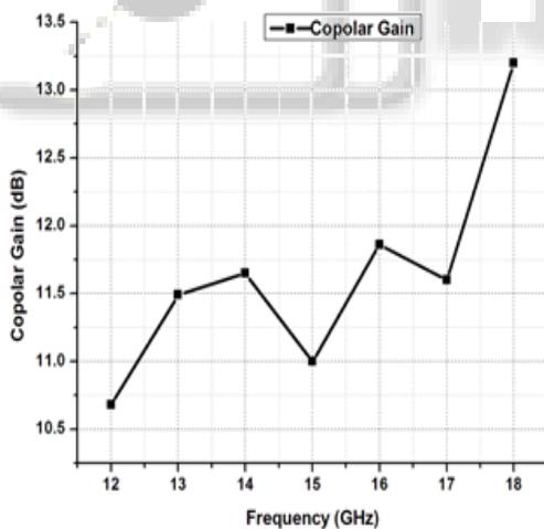
Fig. 12: Frequency vs. Gain graph. It represents the value of gain at different frequency. With the increase in frequency, the value of gain increases.
