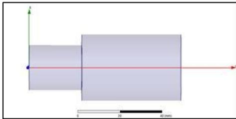
Fig. 2: Design of step discontinuity (a) Side view of design
