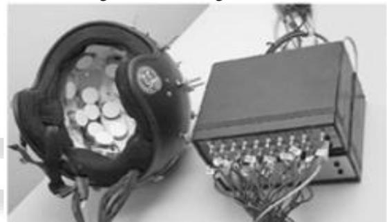
Fig. 4: helmet electrodes placement
