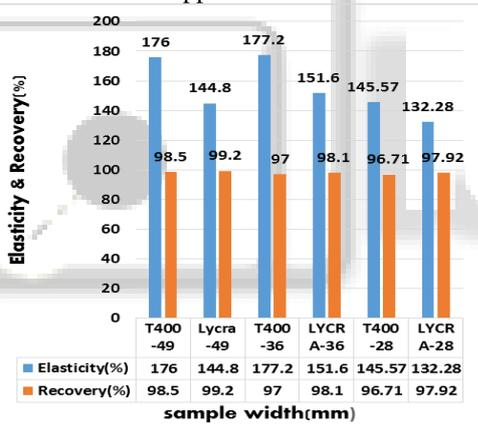
Fig. 2: Graph 2: comparison of Lycra and T-400 sample during elasticity and recovery testing for innerwear tape application.
