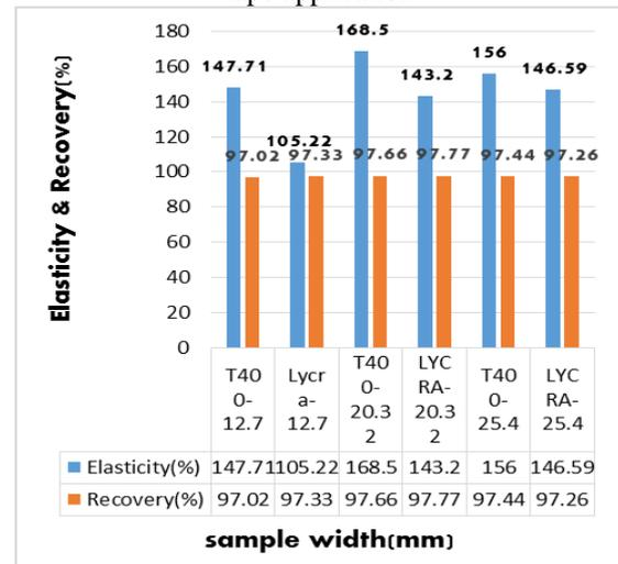
Fig. 3: Graph 3 comparison of Lycra and T-400 sample during elasticity and recovery testing for waist bandages application
