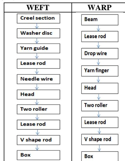
Here show the above passage of JINGYI jyc762/B3 CROCHET machine in case of weft yarn is passes from creel section to box and in case of warp yarn passes from beam to box and finally we can produce the application of narrow wear fabric like some applications innerwear tape and wrist bandages.
