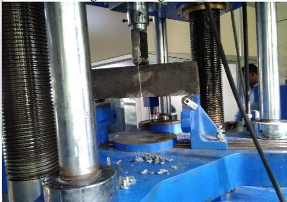
Fig. 7: Beam under loading
