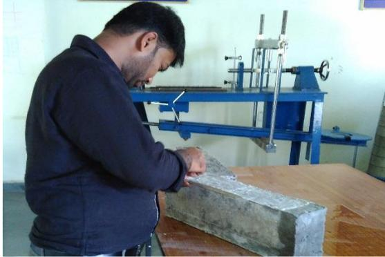
Fig. 6: Marking of beam
