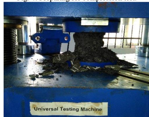
Fig. 5: Specimen failed under load
