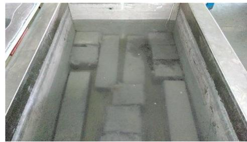
Fig. 3: Curing of specimens in tank
