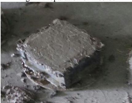
Fig. 2: Concrete filled mould
