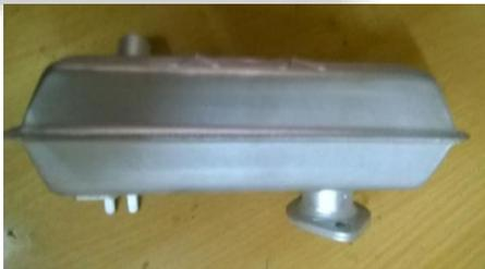
Permanent joints are carried out by riveting, soldering, brazing, welding etc. In silencer, brazing is used for joining parts of the silencer. Brazing is a process of joining two pieces of metals in which a non ferrous filler metal or alloy is introduced between the pieces to be joined. The melting point of the filler metal is above 450<sup>o</sup> c, but lower than the melting temperature of metal.
