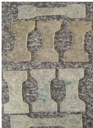
Fig. 3: Epoxy composite specimen
