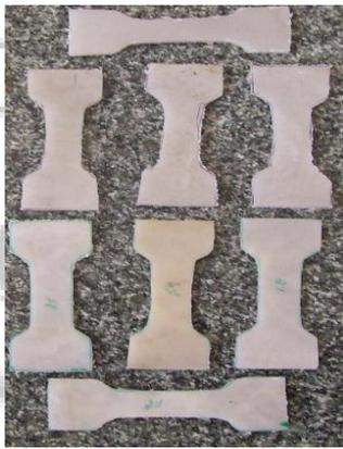
Fig. 2: Polypropylene composite specimen
