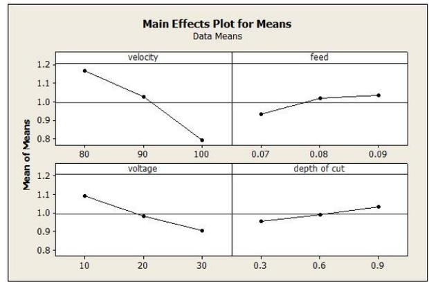
Fig. 13. Graph showing surface roughness at each levels
