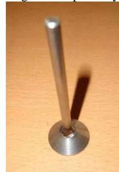
Fig. 4: Piston with piston head
