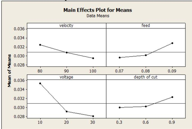
Fig. 11. Graph showing tool vibration at each levels
