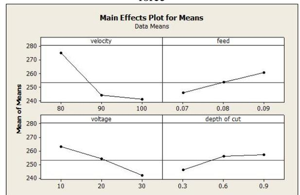
Fig. 15: Graph showing cutting force at each levels
