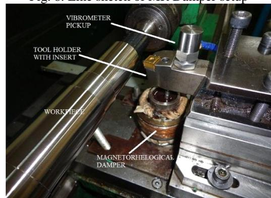
Fig. 9: MR Damper and vibrometer pickup attached to tool holder
