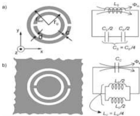
Fig. 1: Topologies of the: (a) SRR and (b) CSRR, and their equivalent-circuit models (ohmic losses can be taken into account by including a series resistance in the model). Grey zones represent the metallization.
