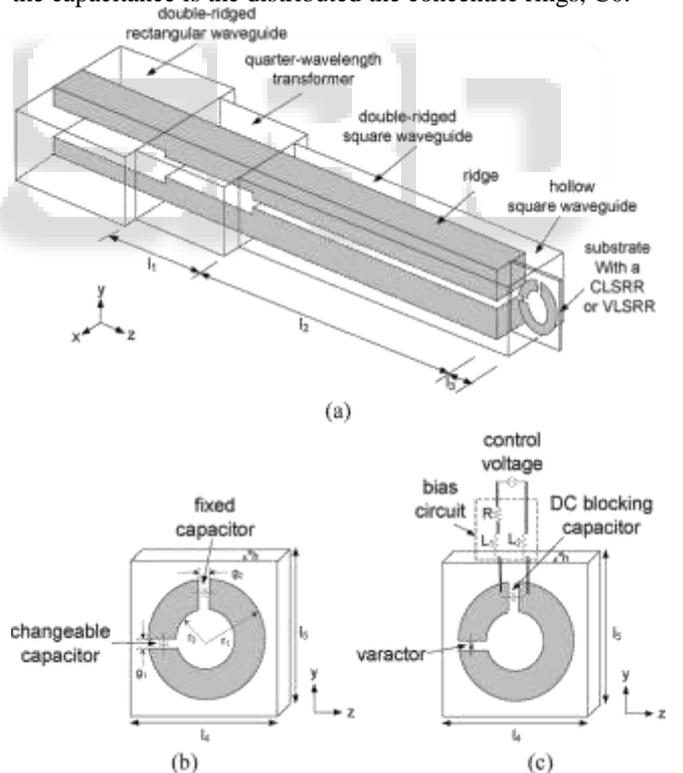
Fig. 4: Geometry of the antenna: (a) Overall view, (b) CLSRR, and (c) VLSRR
