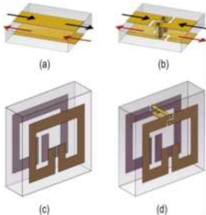
Fig. 5: Geometries of (a) a DSPSL, (b) the DSPSL swap, (c) an SRR in the DSPSL structure, and (d) an ESRR. Dark and red bolts demonstrate the bearings of streams on upper and base strips, individually.
