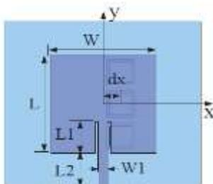
Fig. 3: Configuration of dual band antenna with three CSRRs etched in the ground plane.
