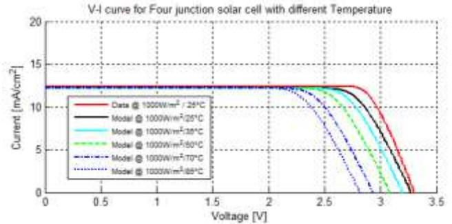
Fig. 6. Temp. Effect on the I-V curve of 4-J solar cell
