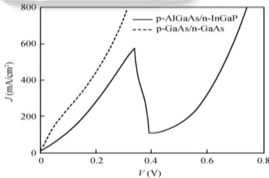
Fig. 2: Characteristics of T-J of solar cell
