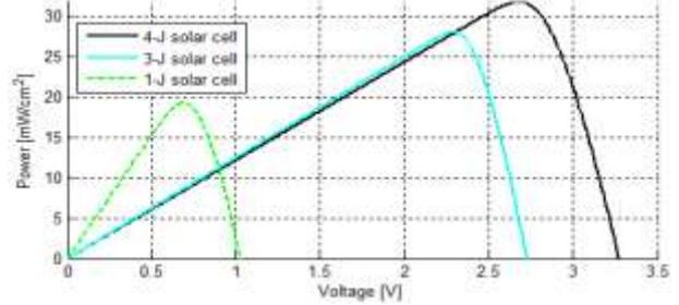
Fig. 11: 4-J, 3-J and single junction P-V curve comparison
