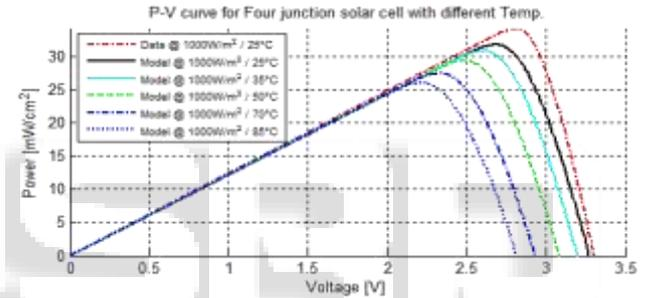
Fig. 7: Temp. Effect on the P-V curve of 4-J solar cell
