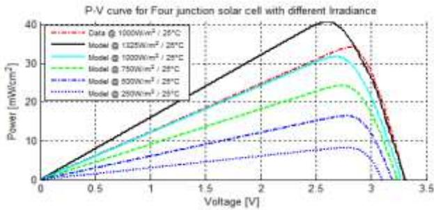
Fig. 9: Irradiance Effect on the P-V curve of 4-J solar cell
