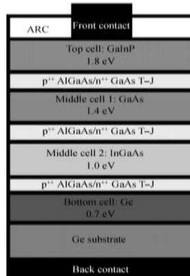
Fig. 1: Four Junction Solar Cell Structure
