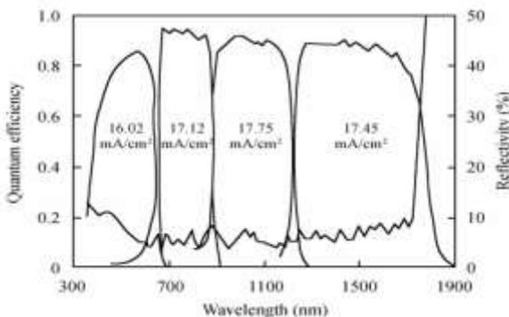
Fig. 3: External quantum Efficiency of Each Sub-cells
