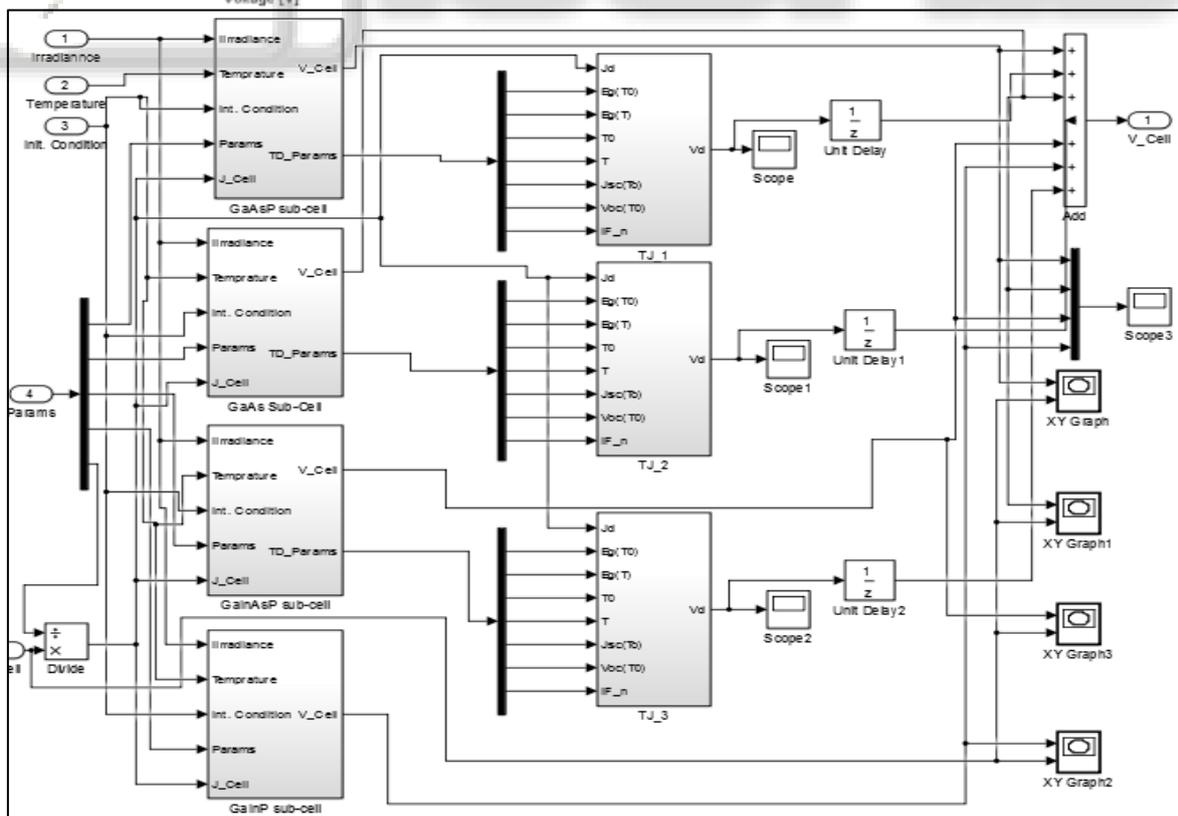
Fig. 12: Main subsystem of 4-j solar cell model implemented in MATLAB/Simulink.
