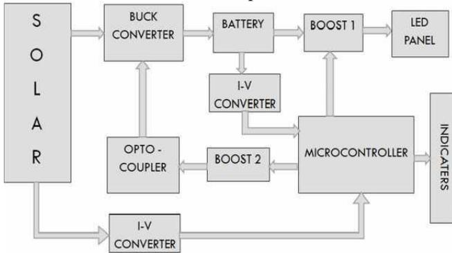
Fig. 1: Block Diagram of MPPT system for Street Lights.
