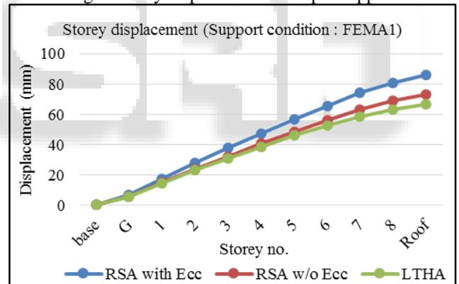
Fig. 7: Storey displacement with FEMA1 support
