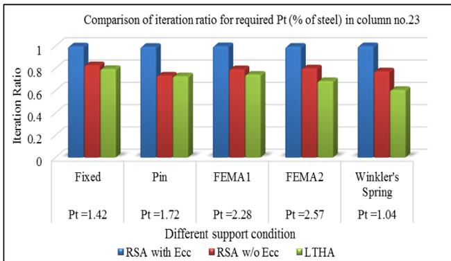
Fig. 17: Comparison of iteration ratio for required Pt (% of steel) in column no.23
