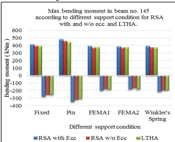
Fig. 12: Max bending moment in beam no. 145
