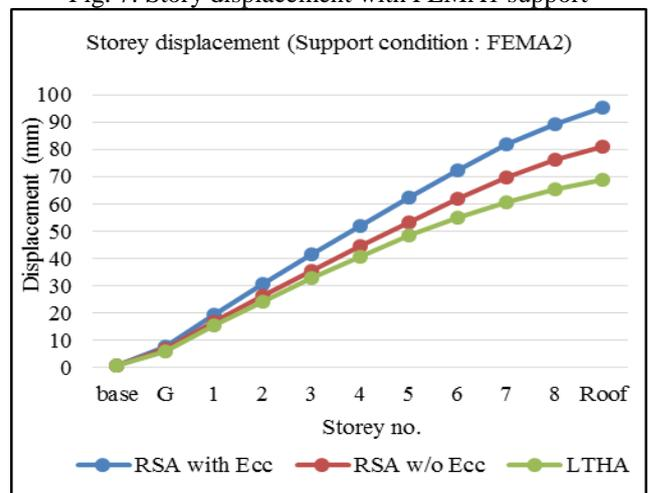
Fig. 8: Storey displacement with FEMA2 support
