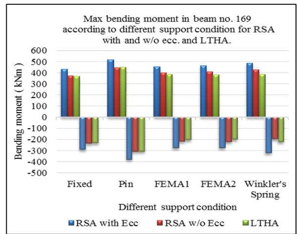
Fig. 13: Max bending moment in beam no. 169
