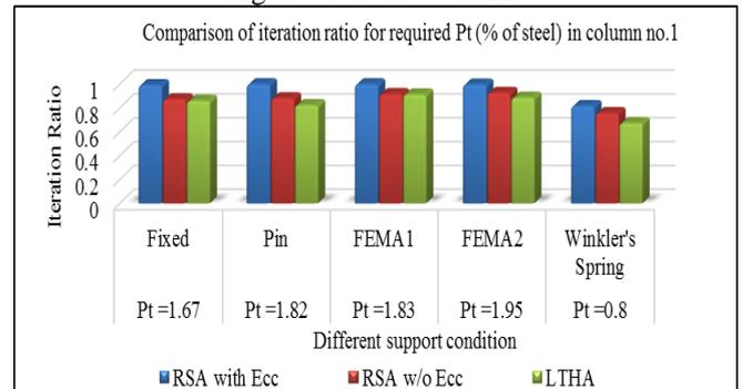
Fig. 15: Comparison of iteration ratio for required Pt (% of steel) in column no.1
