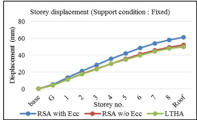
Fig. 5: Storey displacement with fix support
