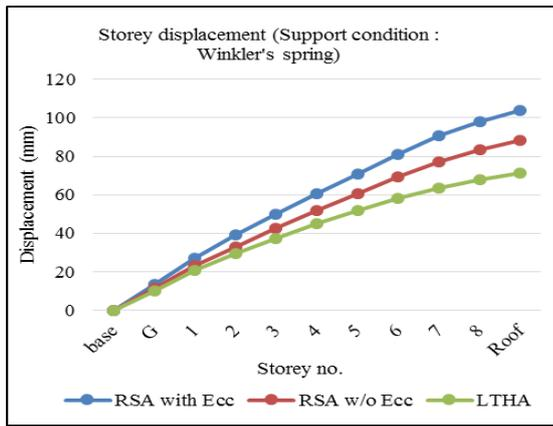
Fig. 9: Storey displacement with Winkler's spring
