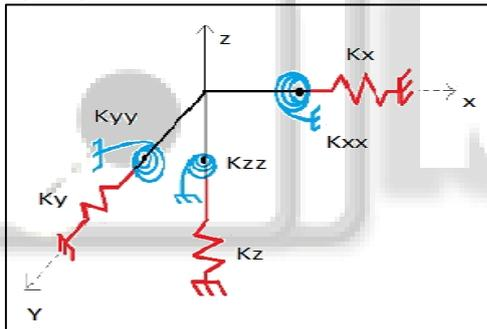
Fig. 3. Equivalent Soil Spring
