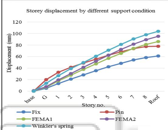
Fig. 10: Storey displacement by RSA with design ecc.
