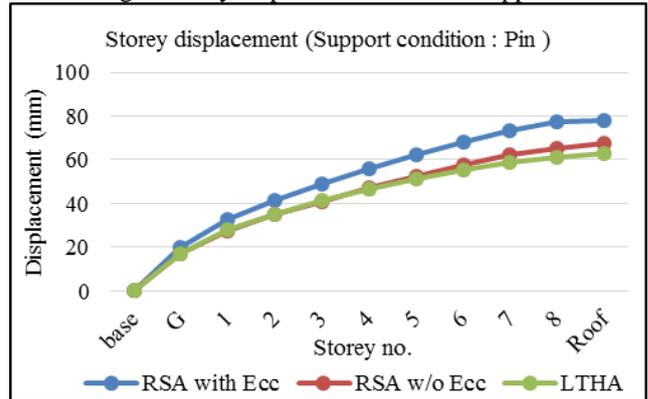
Fig. 6: Storey displacement with pin support
