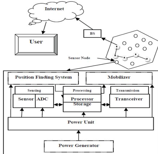
Fig. 1: Architecture of Wireless Sensor Network [2]
