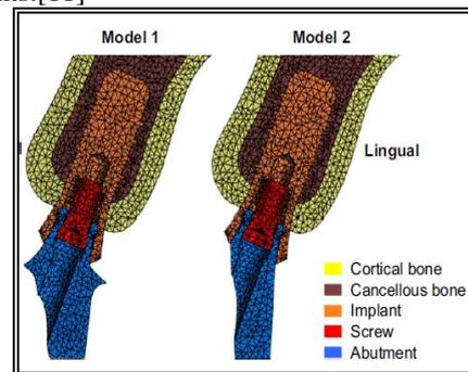
Fig. 4: Finite element models of Model 1 (custom angled abutment design) and Model 2 (conventional angled abutment design).
