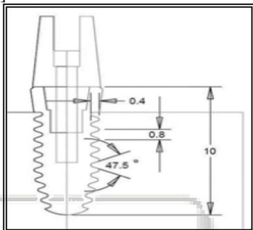
Fig. 2: Dental implant models Type-A.
