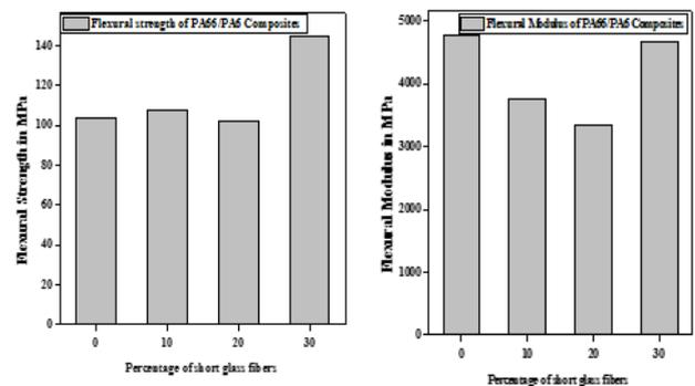
Fig. 6: Flexural behavior of SGF filled PA66/PA6: (a) Flexural strength and (b) Flexural Modulus
