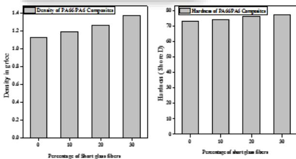
Fig. 4: Variation of properties of SGF filled PA66/PA6: (a) Density and (b) Hardness (Shore D)
