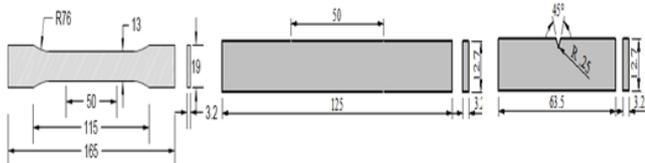
Fig. 3: Specimen standards : (a) ASTM D 638(Tensile Test) (b) ASTM D790 (Flexure Test) and (c) ASTM D256 (Impact Test)
