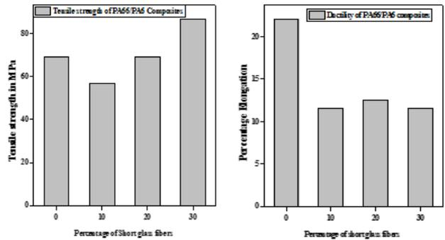
Fig. 5: Tensile behavior of SGF filled PA66/PA6: (a) Tensile strength and (b) % Elongation
