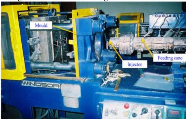
Fig. 1: Injection Molding Machine
