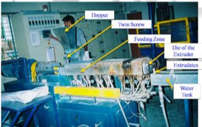
Fig. 1: Barbender Co- Rotating Twin Screw Extruder
