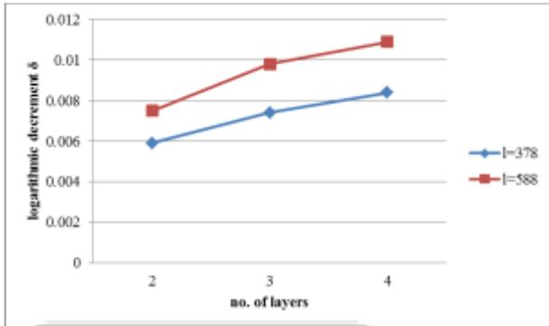
Fig. 8: variation of logarithmic decrement with respect to number of laminates for beams of different lengths.
