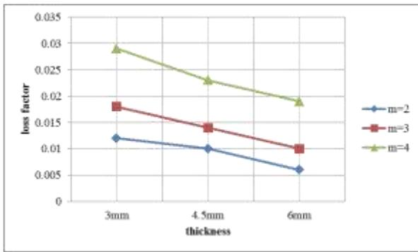
Fig. 7: variation of loss factor with respect to thickness of laminates for different number of laminates for  $m=2$  and  $m=3$ .
