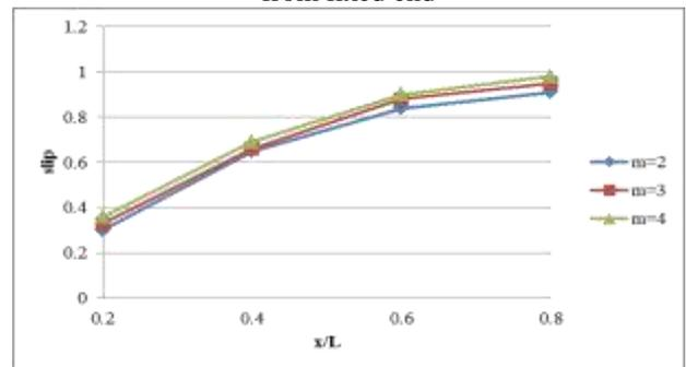
Fig. 5: Variation of relative slip with axial distance from free end for specimen of different number of layers.
