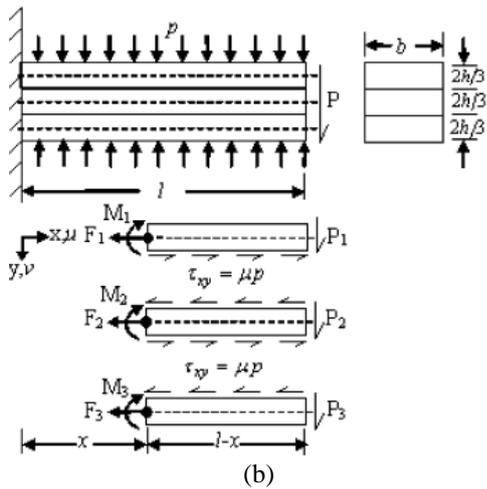
Fig. 1(a): Three layered tack welded cantilever beam model.
