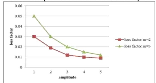
Fig. 6: variation of loss factor with respect to amplitude for m=2 and m=3.
