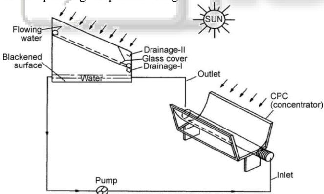
Fig. 8: Solar still integrated with CPC concentrator
