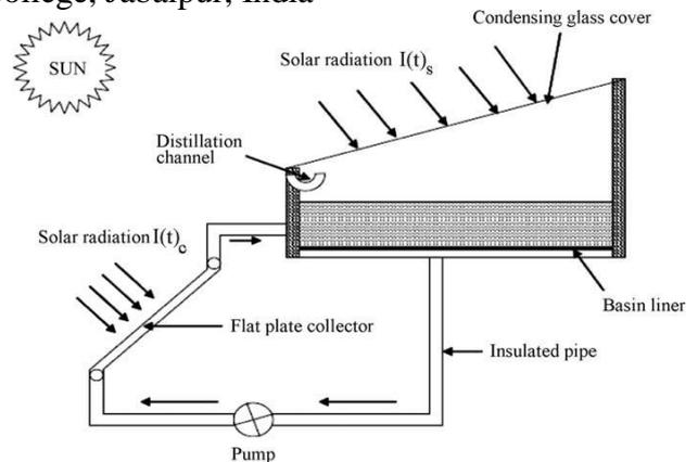
Fig. 1: Layout of active solar still
