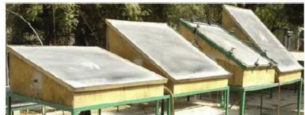
Fig. 3: Solar stills with different inclinations
