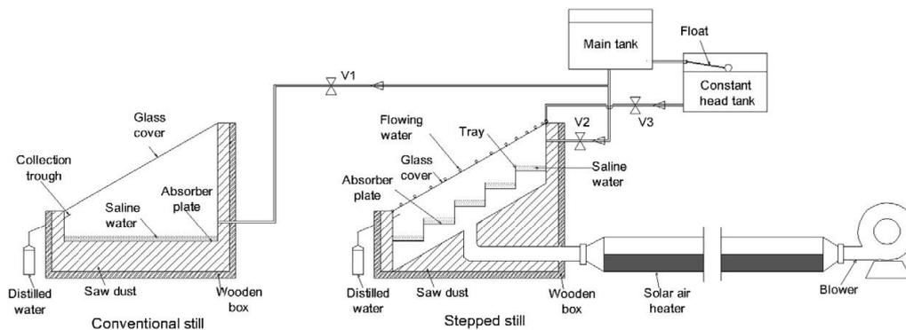
Fig. 10: Stepped solar still coupled with a solar air-heater.
