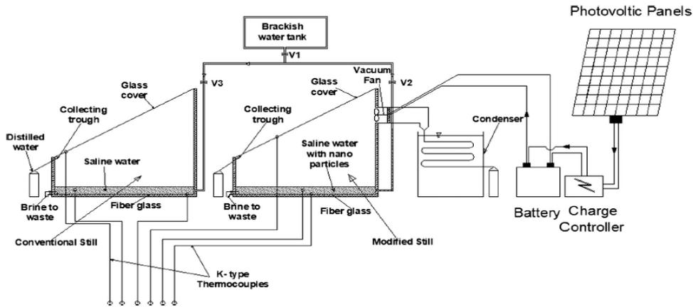
Fig. 7: Solar Still Integrated With External Condenser
