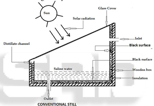
Fig. 2: Layout of active solar still
