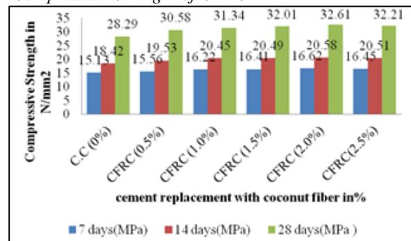
Fig 8: Compressive strength values of C.C and CFRC at 3, 7 and 28 days
