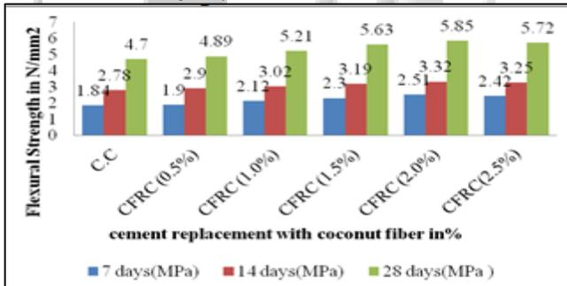
Fig 10: Flexural strength values of C.C and CFRC at 7, 14 and 28 Days
