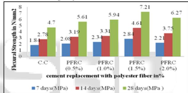
Fig 7: Flexural strength values of C.C and PFRC at 7, 14 and 28 Days
