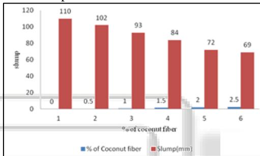
Fig 4: Variation of Slump in Coconut fiber
