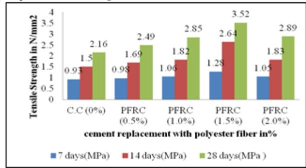
Fig 6: Split tensile strength values of C.C and PFRC at 7, 14 and 28 Days
