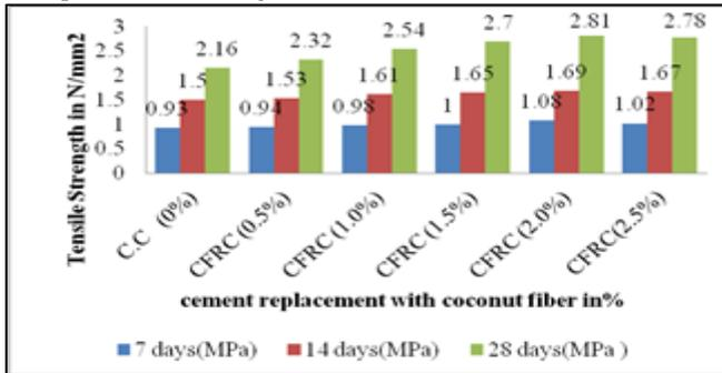
Fig. 9: Split tensile strength values of C.C and CFRC at 7, 14 and 28 Days
