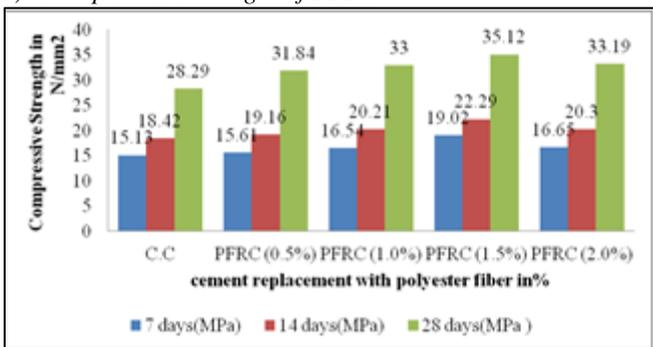
Fig. 5: Compressive strength values of C.C and PFRC at 7, 14 and 28 Days
