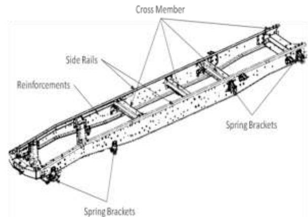
Fig. 1: Heavy Vehicle Chassis Frame
