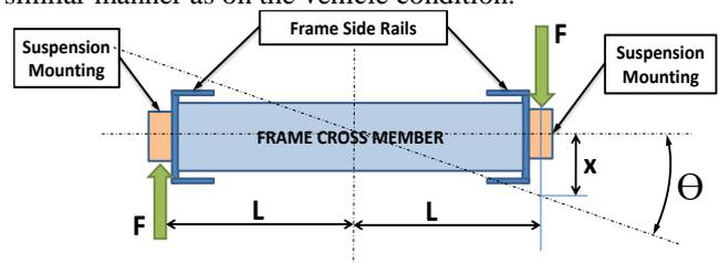
Fig. 5: Chassis frame torsion stiffness loading.
