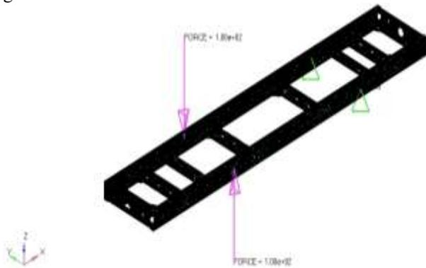
Fig. 6: Boundary and loading condition at wheel base.
