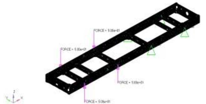
Fig. 8: Boundary and loading condition at spring brackets.
