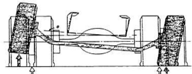
Fig. 2: One wheel of a axle on road bump - Torsion Load [4]
