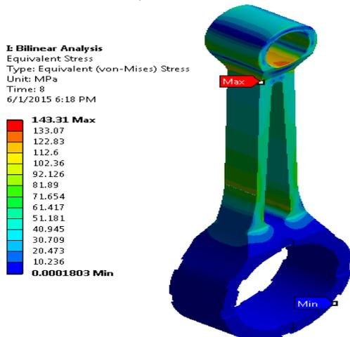
Fig. 7: Bi Linear Static Analysis
