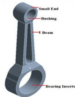
Fig. 1: Schematic representation of connecting rod
