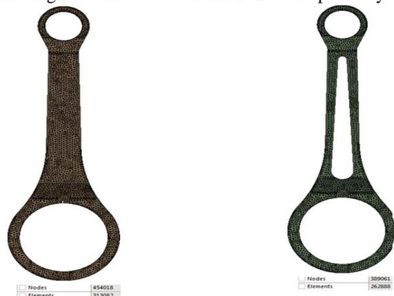
Fig. 4: Finite Elements Models
