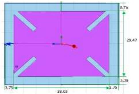
Fig. 2: Top view of the meandered corner micro strip patch antenna (all dimensions are in mm).
