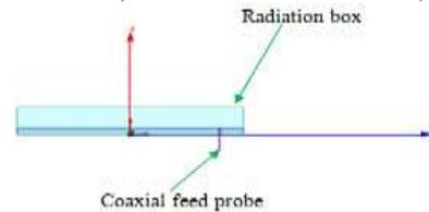
Fig. 3: Side view of the antenna showing the coaxial feed point and radiation box.
