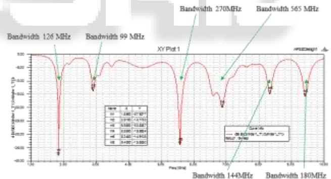
Fig. 4: Return Loss (S11) of the Antenna.
