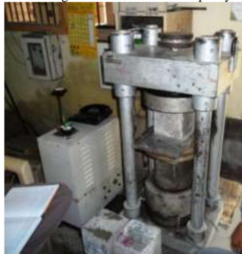
Fig. 3: Compression Test
