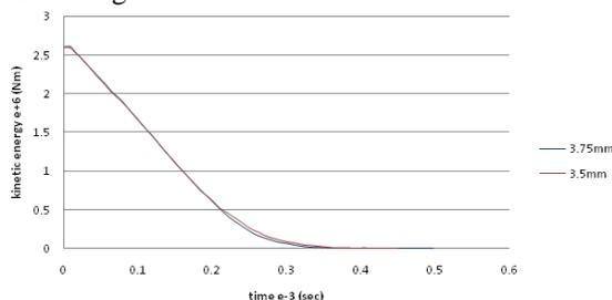
Fig. 15: kinetic energy variation of blade speed (27350 rpm) with time on flat geometry.
