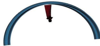
Fig. 3: Blade with containment ring with convex curve geometry.
