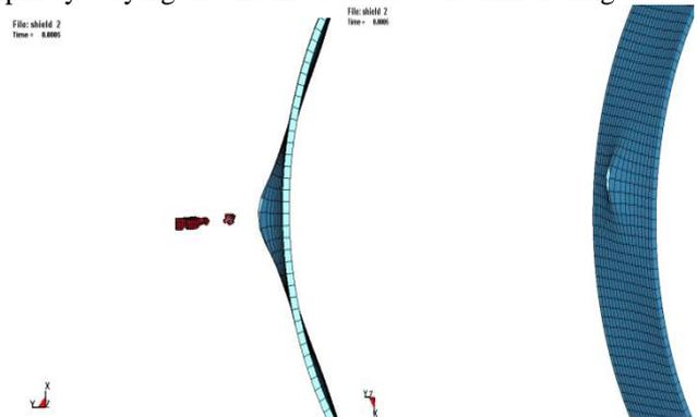
Fig. 12: condition of the containment ring at 3.5 mm and 3.75 mm thickness.
