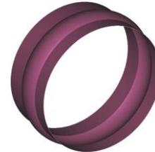
Fig. 1: Fan containment ring with radial convex curve in its geometry.
