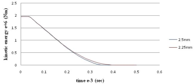
Fig. 16: kinetic energy variation of blade speed (23500 rpm) with time on convex curve geometry.
