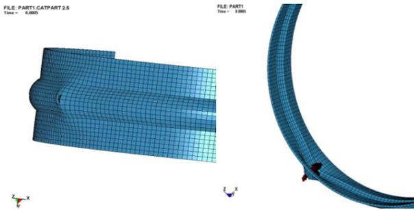
Fig. 13: condition of the containment ring at 2.5 mm and 2.25 mm thickness.
