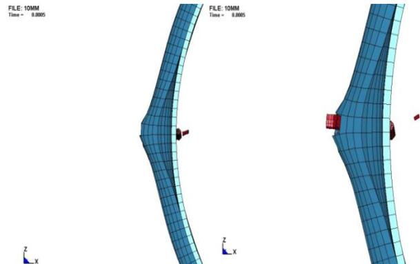
Fig. 11: condition of the containment ring at 10 mm thickness.
