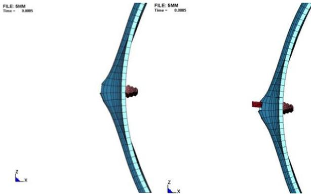
Fig. 6: condition of the containment ring at 5 mm thickness.
