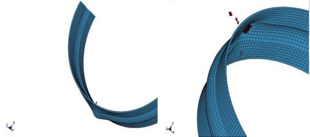
Fig. 8: condition of the containment ring at 7 mm thickness.
