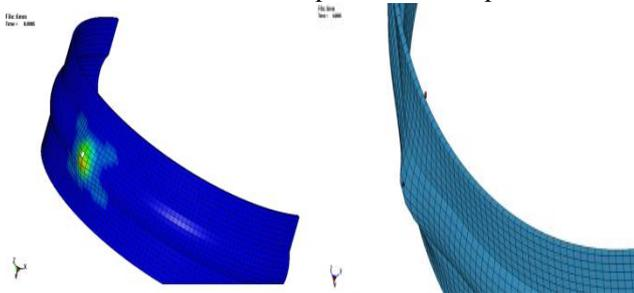
Fig. 7: condition of the containment ring at 6 mm thickness.
