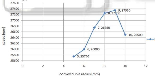
Fig. 14: speed of blade vs. curvature of the containment ring.
