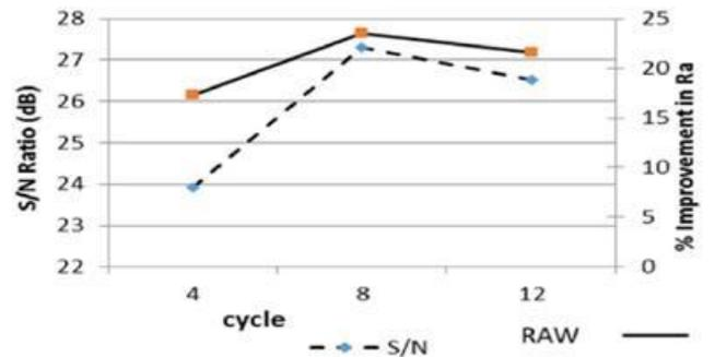
Fig, 3 Effect of Number of Cycle on Percentage Change in Surface Roughness
