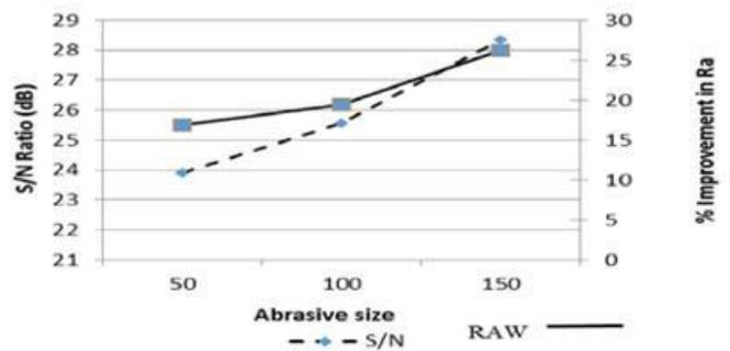
Fig, 2 Effect of abrasive size on percentage change in surface roughness
