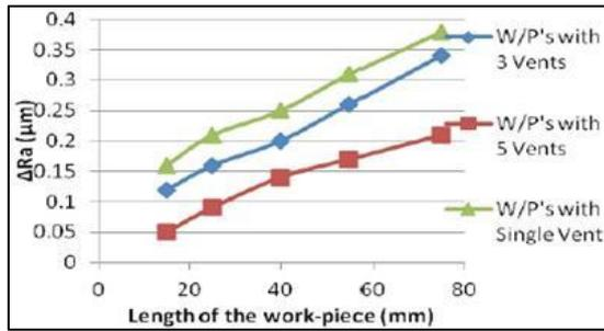
Fig.4 Effect of different vent considerations in work-pieces of varying lengths on  $\Delta Ra$
