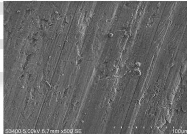
Fig. 5: Microstructure of aluminium reinforced with 4% silicon carbide.
