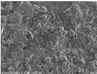
Fig. 7: Microstructure of aluminium reinforced with 8% silicon carbide.
