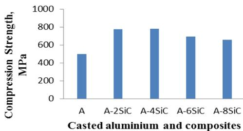
Fig. 2: Chart showing compression strength of aluminium reinforced with silicon carbide.
