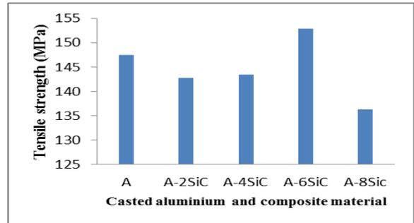
Fig. 3: Chart showing the tensile strength of aluminium reinforced with silicon carbide.
