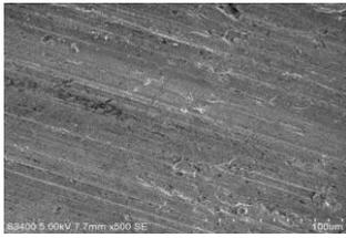
Fig. 8: Microstructure of cast aluminium alloy 6061
