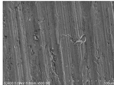
Fig. 6: Microstructure of aluminium reinforced with 6% silicon carbide.
