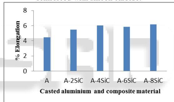
Fig. 4: Chart showing % elongation of aluminium reinforced with silicon carbide.
