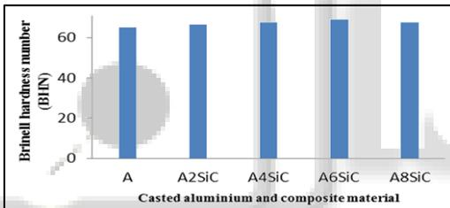
Fig. 1: Chart showing (BHN) of aluminium reinforced with silicon carbide
