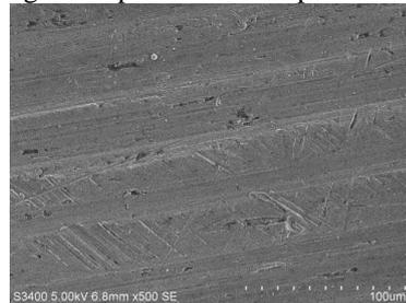
Fig. 4: Microstructure of aluminium reinforced with 2% silicon carbide.
