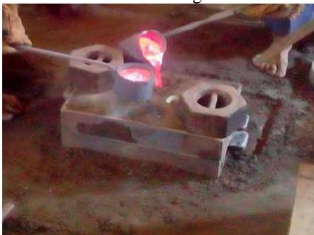
Fig. 3: Pouring of molten Al-SiC composite into the mould.
