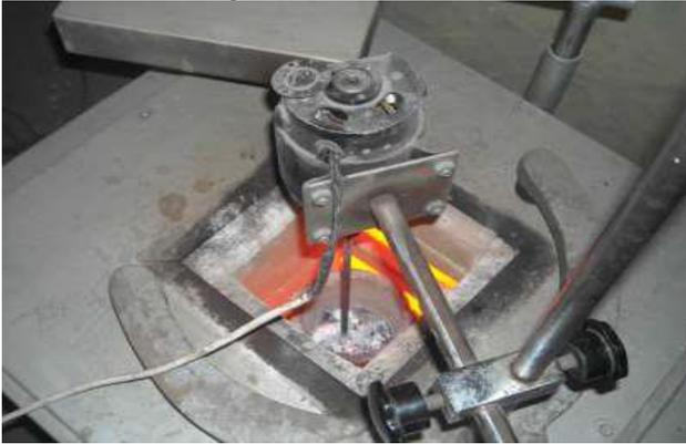
Fig. 1: Stir Casting Set Up.
