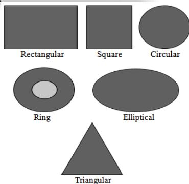
Fig. 1: Different basic patch structure
