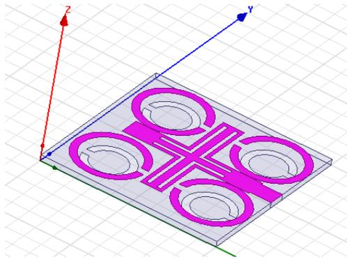
Fig. 3: Design of proposed metamaterial structure at the height of 1.57 mm from ground plane.
