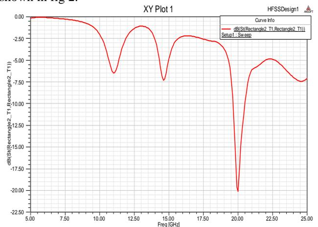
Fig. 2: Simulation of return loss and bandwidth of MPA
