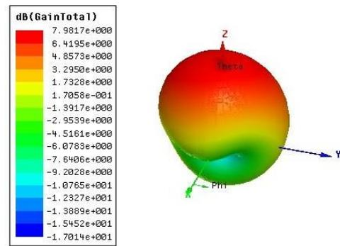
Fig. 7: Antenna Gain of MPA with proposed metamaterial structure
