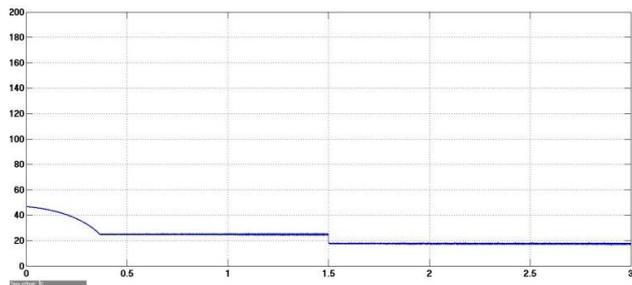
Fig. 6: Inverter bus voltage of BLDC motor by using ANFIS controller
