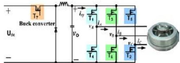
Fig. 2: Buck converter-based BLDCM drive system block diagram.
