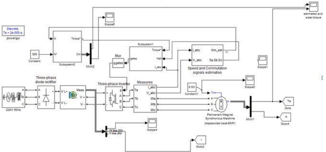
Fig. 4: Simulink diagram for speed and torque of BLDC motor by using ANFIS controller
