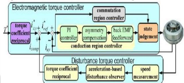
Fig. 1: Quickend torque control scheme block diagram.
