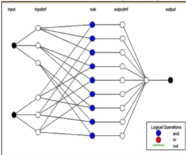
Fig. 3: Structure of ANFIS controller
