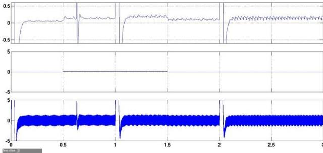
Fig. 11: Performance during sudden change in speed by using PI controller based BLDC motor
