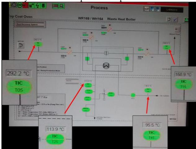
Fig. 6: Schematic view of heat recovery system on ECO screen Showing actual readings of water & exhaust gases.
