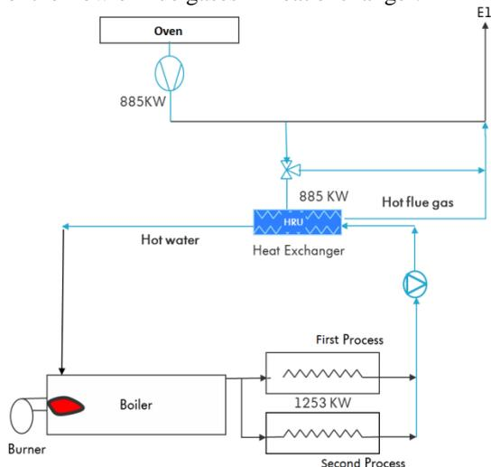
Fig. 1: Exhaust along with Heat exchanger
