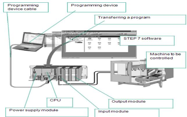
Fig. 4: Communication between PC and PLC
