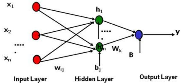
Fig. 2: Multilayer Perception Architecture with Hidden Layers
